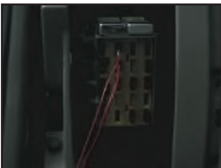
13. Connect the red wire to the constant 12v source. This source will have 12v at all times.
